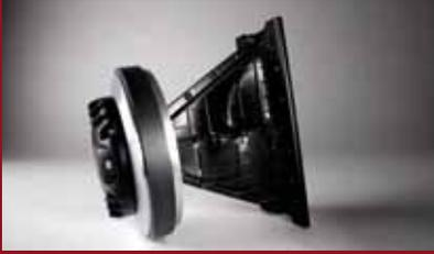
The CD850 large format compression driver delivers one of the key advantages of the HDL 20-A, the 3" voice coil allows a crossover point of 800Hz and therefore almost all of the vocal range can be produced by this driver. This allows better coverage and dispersion control, and superior efficiency.
