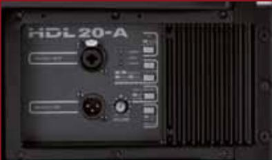
The easy to access controls on the back of the speaker allow a number of simple optimisations to be carried out at the flick of a switch: two possible HF settings, four possible cluster configurations; a special EQ setting for high curved configurations and an Indoor Correction EQ.
